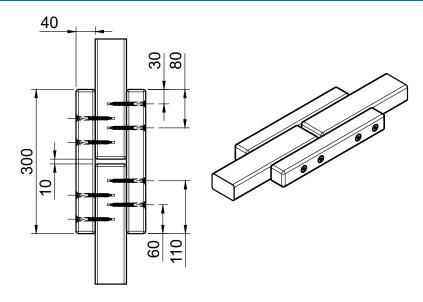
Joiner fixing requires 75 mm stainless steel bugle screws Enduroplank<sup>TM</sup> fixing requires 100 mm stainless steel bugle screws
