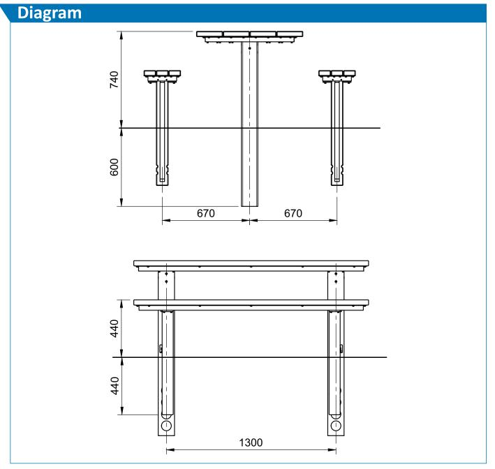
All dimensions are in millimetres (mm) unless specified.
