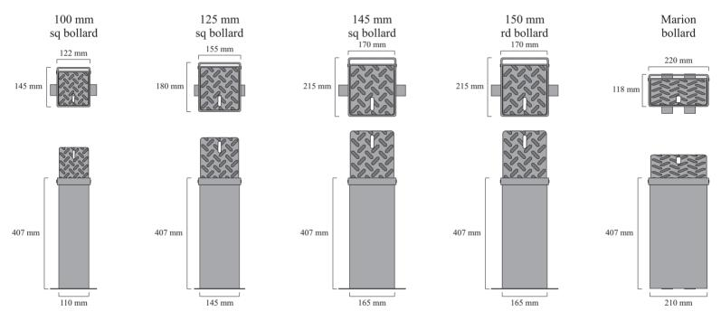
Made from galvanised steel, the hinged sleeves are highly durable and help create a flexible solution for your boundary.
